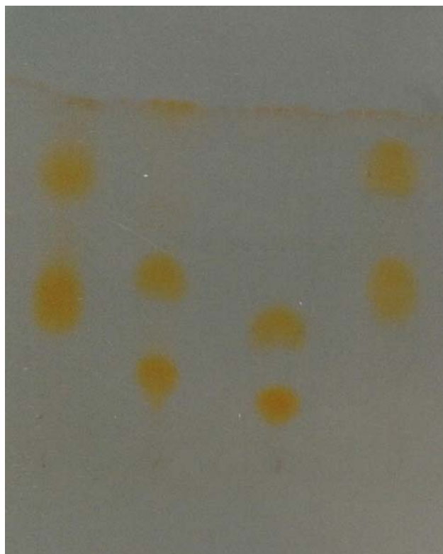
Fig. 2 Chromatogram obtained by normal phase TLC showing separation of the diastereomers of DL-amino acids derivatized with FDNP-L-Phe-NH 2 . From left to right norvaline, aminoadipic acid, cysteic acid and isovaline. The upper spot is the D diastereomer and the lower spot is the L diastereomer. The mobile phase was phenol-water, 3:1, and the distance to the solvent front was 5.0 cm
